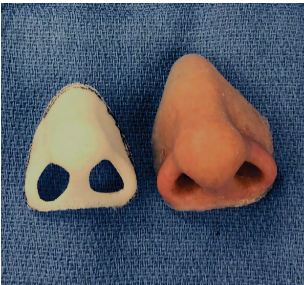
Fig. 2. Three-dimensional printed custom PPE scaffold (left) compared to the silicone prosthesis upon which the scaffold was based.
